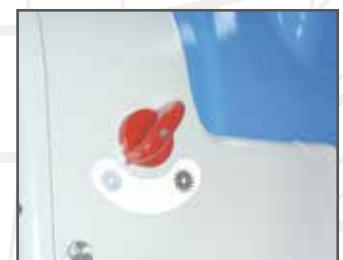
*The “SCU” device is operated by means of a manual switch located in the bottom front part of the guard. By means of the switch, the tool to be used can be selected: blade for cutting , cutter for grooving (in the case of the KGS/GMC 180 CN. model the switch is operated by the programming unit). The grooving cutter is activated by means of a pneumatic cylinder.*
